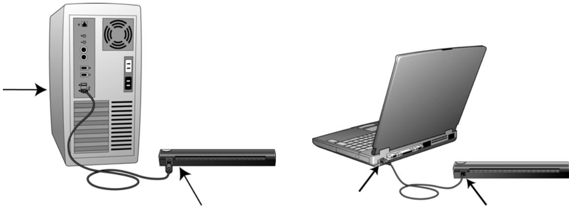
If the plug does not attach easily, make sure that you are plugging it in correctly. Do not force the plug into either connection.
