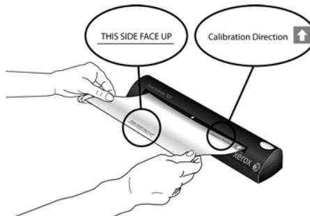
6. The scanner will pull the calibration page through the scanner. The page will move back and forth as the scanner calibrates for the difference between dark and light.
