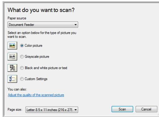
1. On the scan window, click **Adjust the quality of the scanned picture**.
